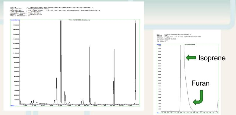
DB-624, length 60 m, I.D. 0.25 mm, 1.4 µm film.
