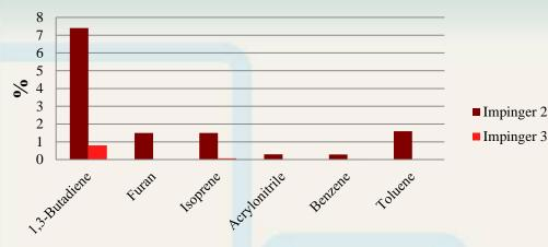
With 10 ml of trapping solution in front impinger, 1,3 butadiene was trapped with 93% efficiency (intense smoking)
