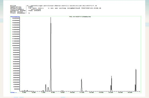
Rxi-1ms, length 60 m, I.D. 0.25 mm, 1.0 µm film.
