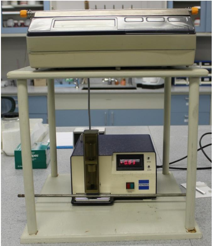
Applied load of DHT tested = ~298 g
