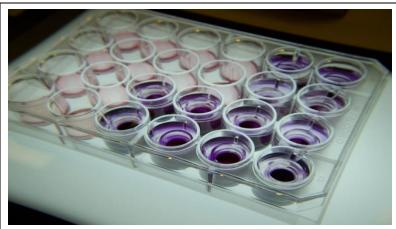
Individual tissues are placed into wells containing unreduced 3-(4,5-dimethylthiazol-2-yl)-2,5diphenyltetrazolium bromide (MTT) solution
