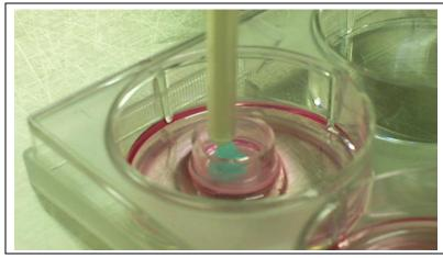
Dosing of aqueous or semi-viscous test chemicals or formulations is performed with a positive displacement pipette
