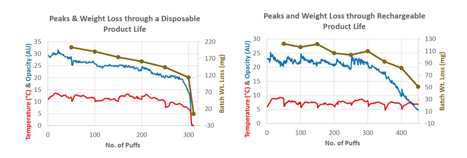
For the disposable, it can be seen that the production of aerosol is abruptly terminated as the battery expires after 311 puffs, whereas for the rechargeable, the puff temperature is maintained (since the battery was replaced) but that after about 300 puffs the production of aerosol gradually declines as the e-juice runs out.
