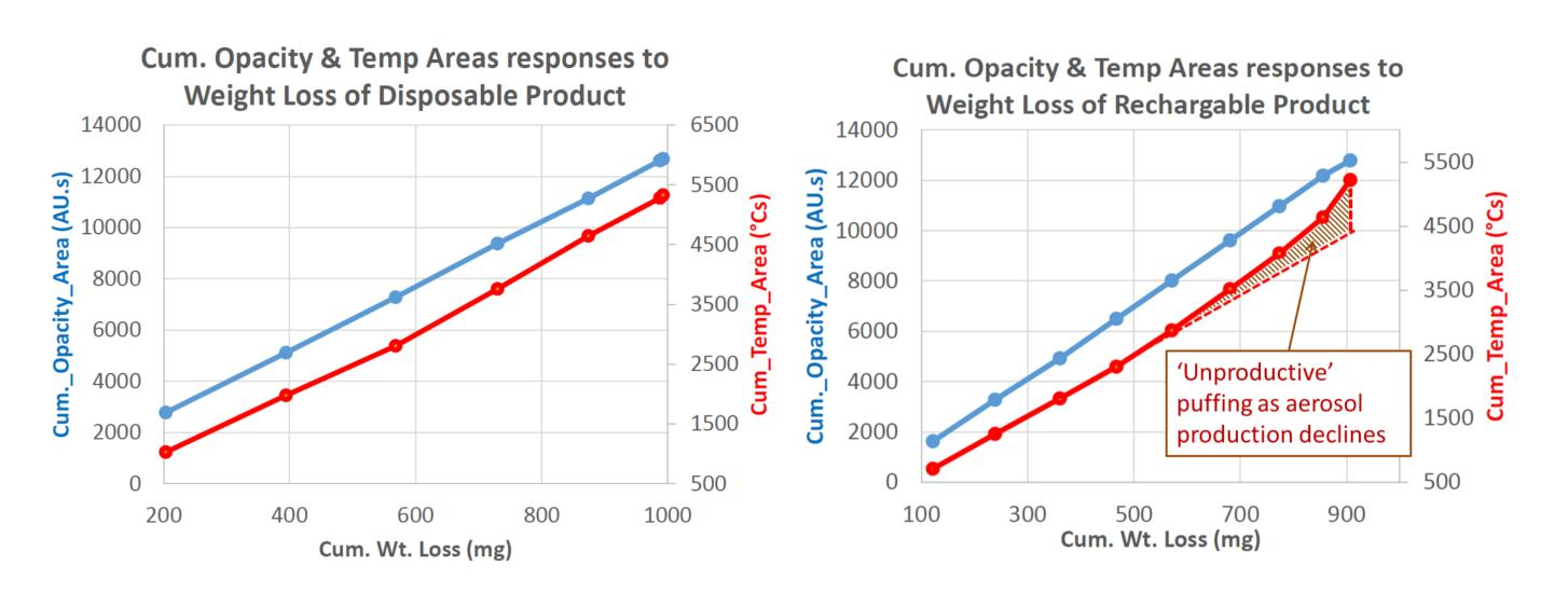
The aerosol plots appear to be linear while the temperature plots are both somewhat curved, particularly for the rechargeable product. This equates to the less productive puffs towards end-of life as the e-juice runs out.
