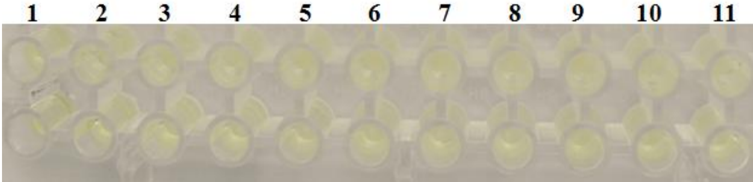
R. solanacearum growth inhibition tests by mancozeb on 96-well plate (1-11:100 mg/L -50-25-12.5-6.25-3.13-1.56-0.78-0.39-0.2-ck)
