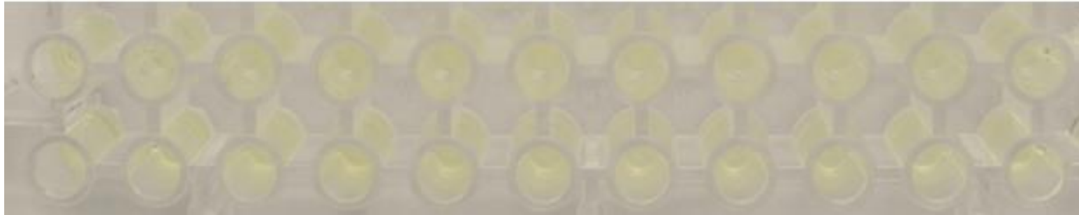
R. solanacearum growth inhibition tests by calcium oxide on 96-well plate (1-11:1250 mg/L -625-313-156-78-39-18.5-9.25-4.6-2.3-ck)
