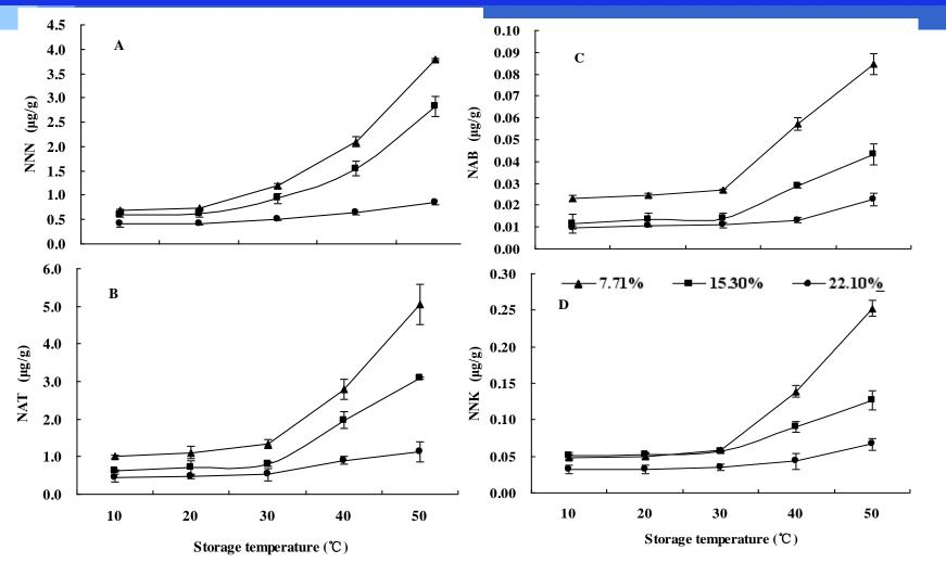
When storage temperature exceeded 30°C, significant differences (P<0.01) were observed both in individual and total TSNA contents among samples for tobaccos with different moisture contents.
