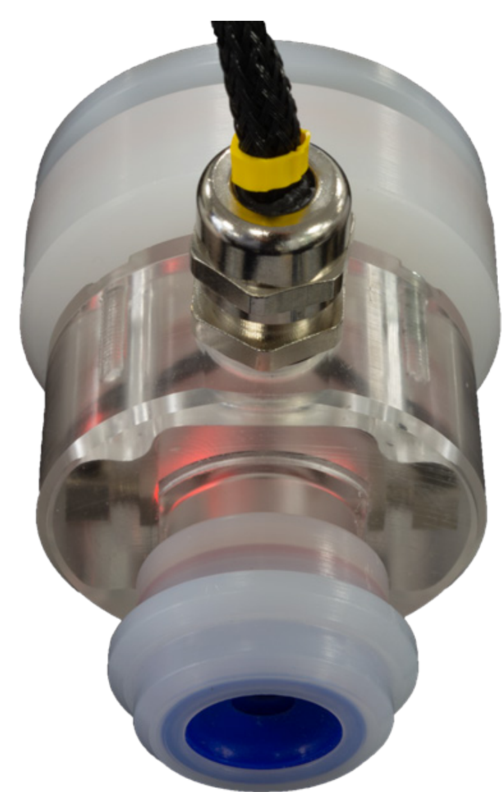
Fig. 3 Cambridge Filter Holder with opacity sensor
