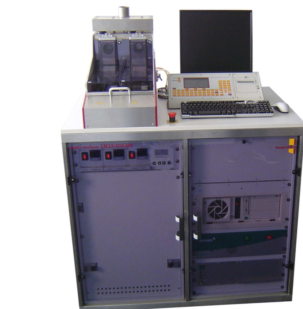
Figure 1: Experimental setup with the commercial available LM2X Smoke Analyzer from Borgwaldt KC and Photonion GmbH (Germany)
