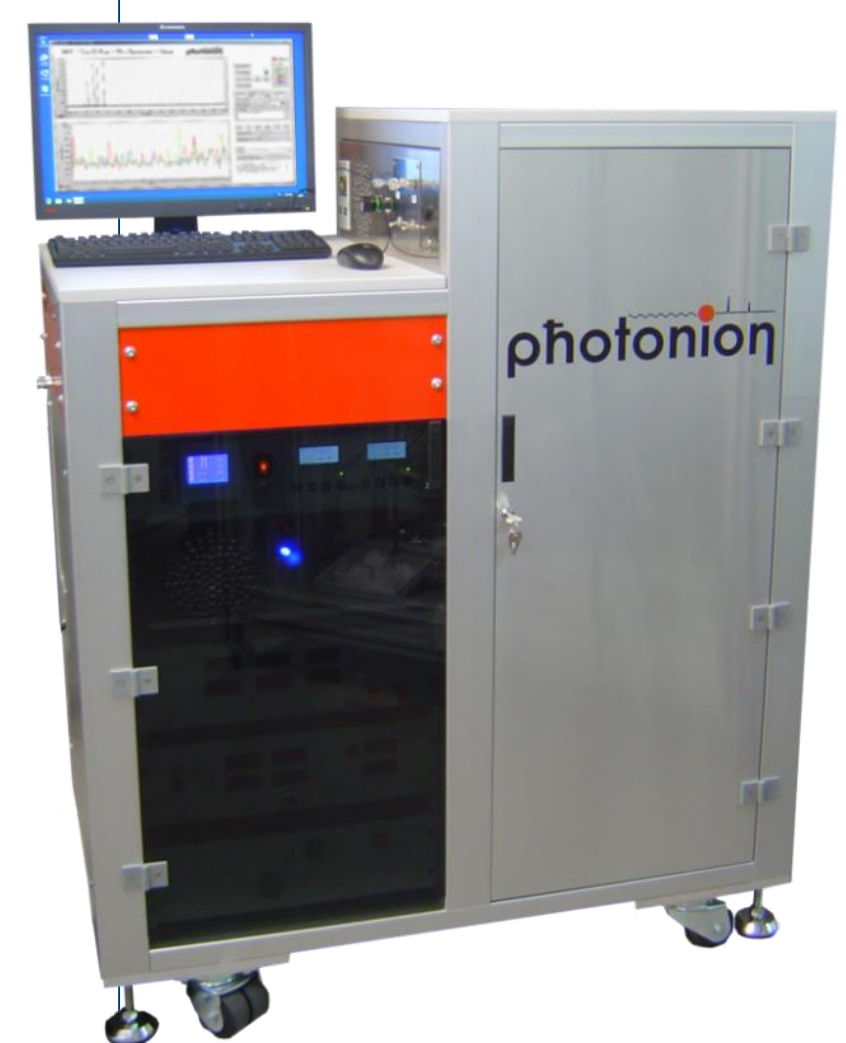
Figure 1: Experimental setup with the commercial available SPI/REMPI ToF-MS of Photonion GmbH (Germany)
