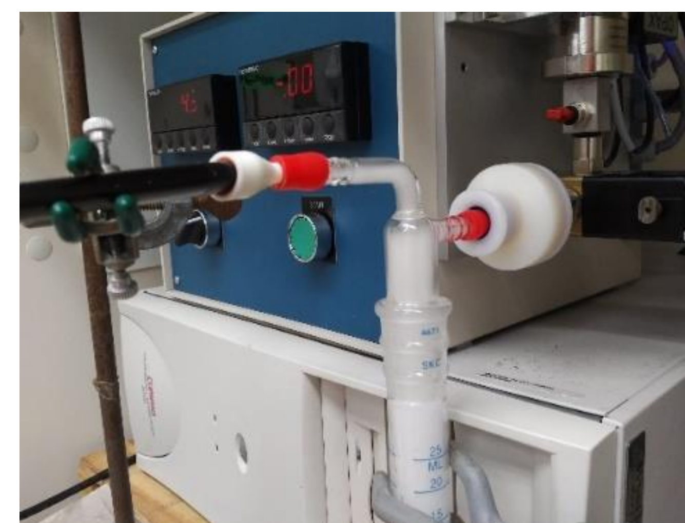
Figure 3. Experimental setup for passing e-cigarette aerosol through an impinger filled with a spin-trapping solution.
