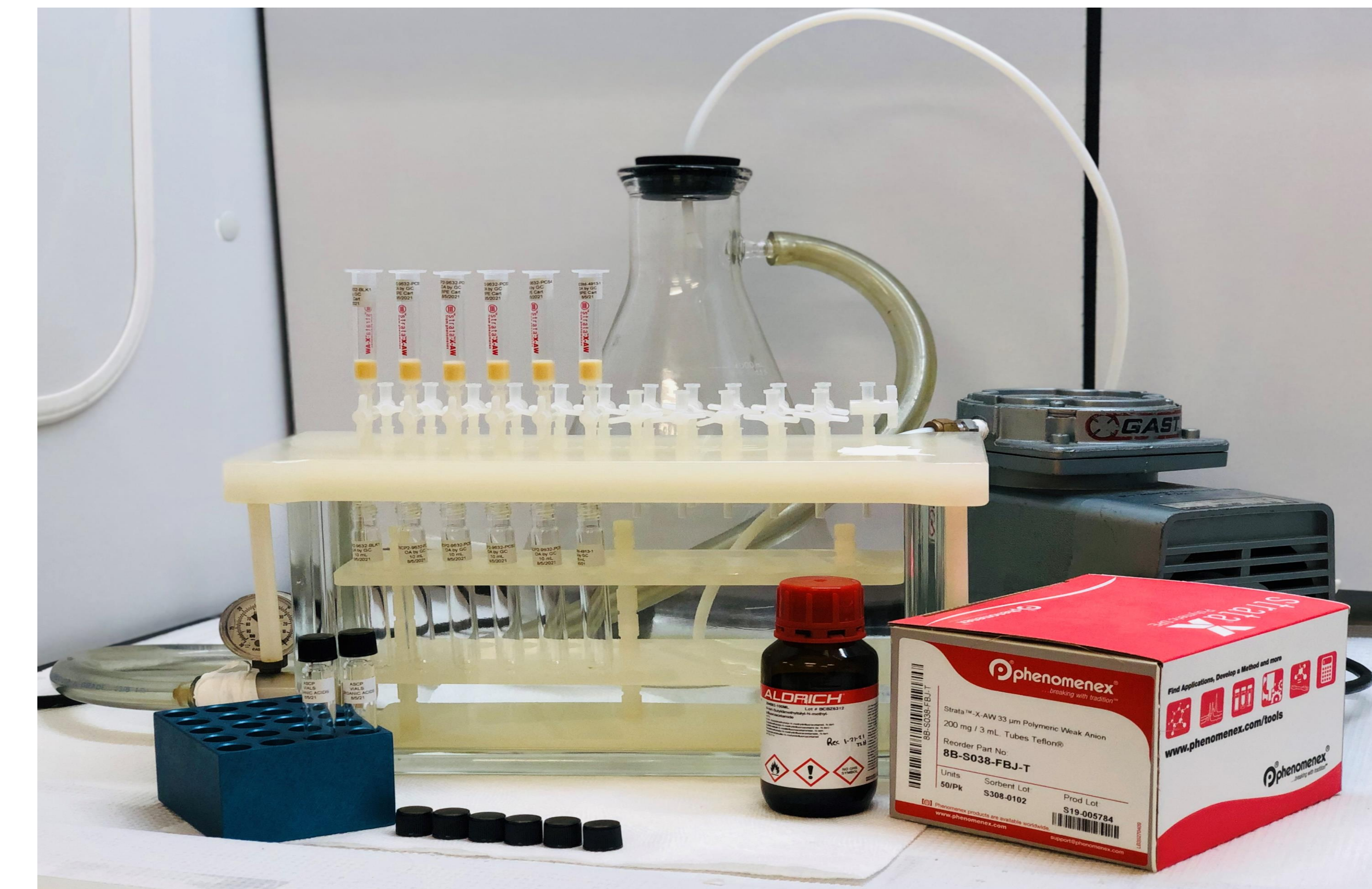
Figure 3 – Vacuum manifold, Strata X-AW anion exchange cartridges, MTBSTFA reagent, and extract.
