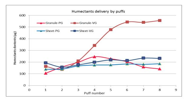
Both PG and VG show a more stable delivery pattern from substrate material in sheet form;
