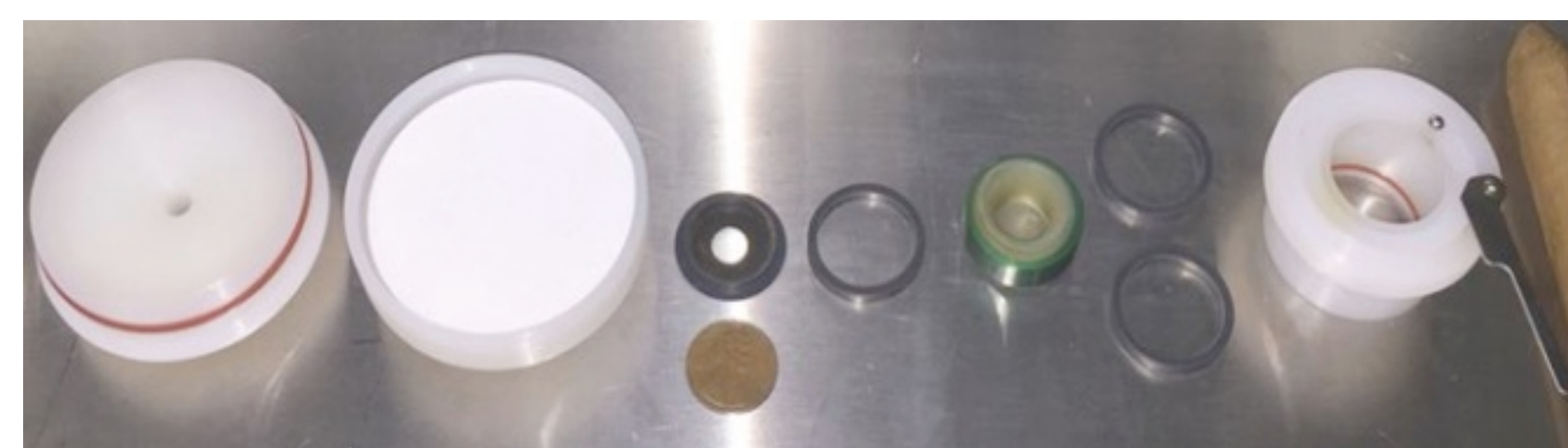
Figure 2. The components of the CORESTA cigar adaptor (penny shown for scale)
