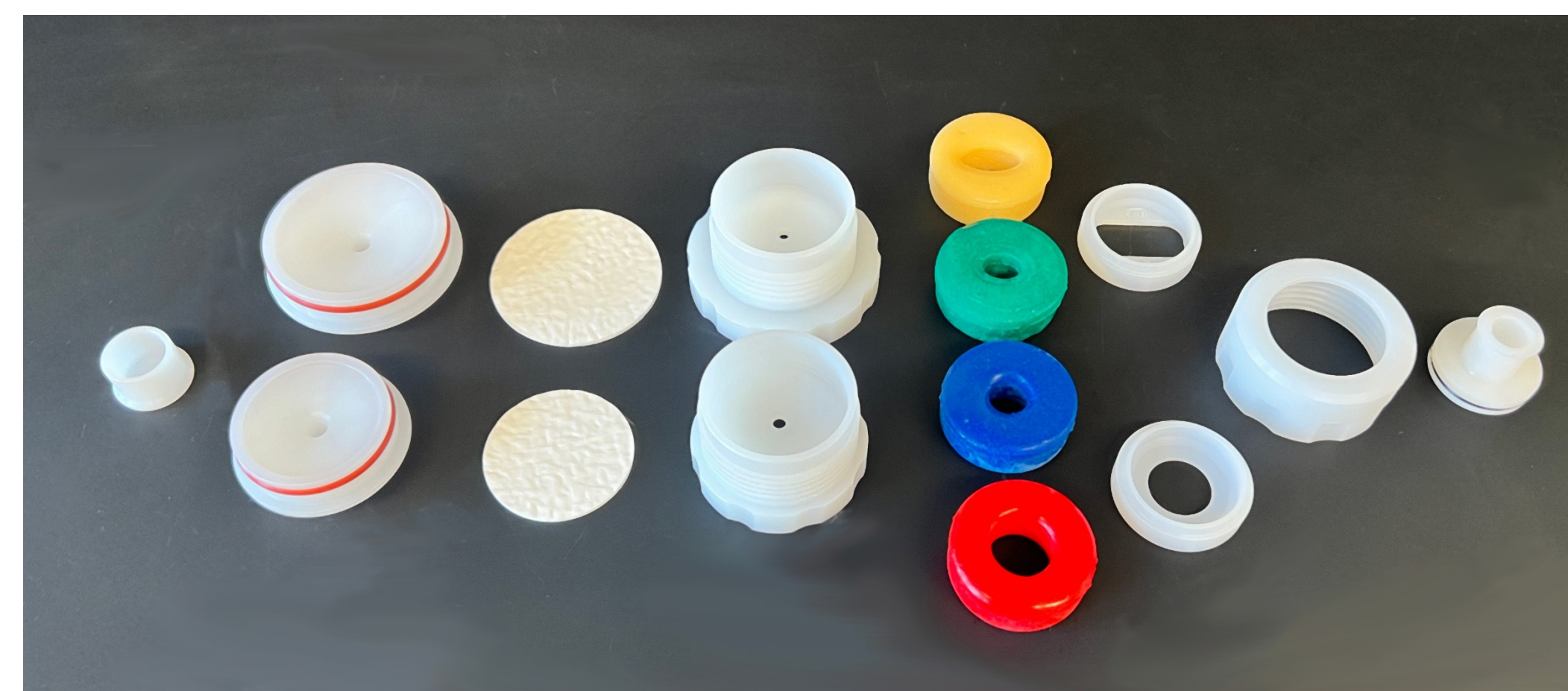
Figure 1. The rigid and flexible components of the 55 mm diameter (top) and 44 mm diameter (bottom) USMA. (Left to right): back of filter holder, filter pad, base, flexible ferrules, compression plates, and threaded cap.
