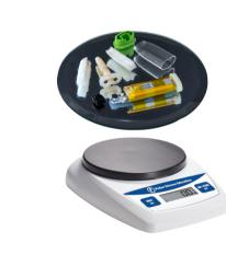
Dried components re-weighed to determine total liquid removed
