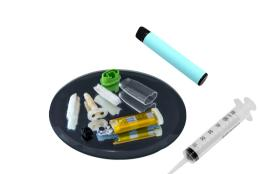
E-cigarette disassembled, washed and as much e-liquid as possible removed
