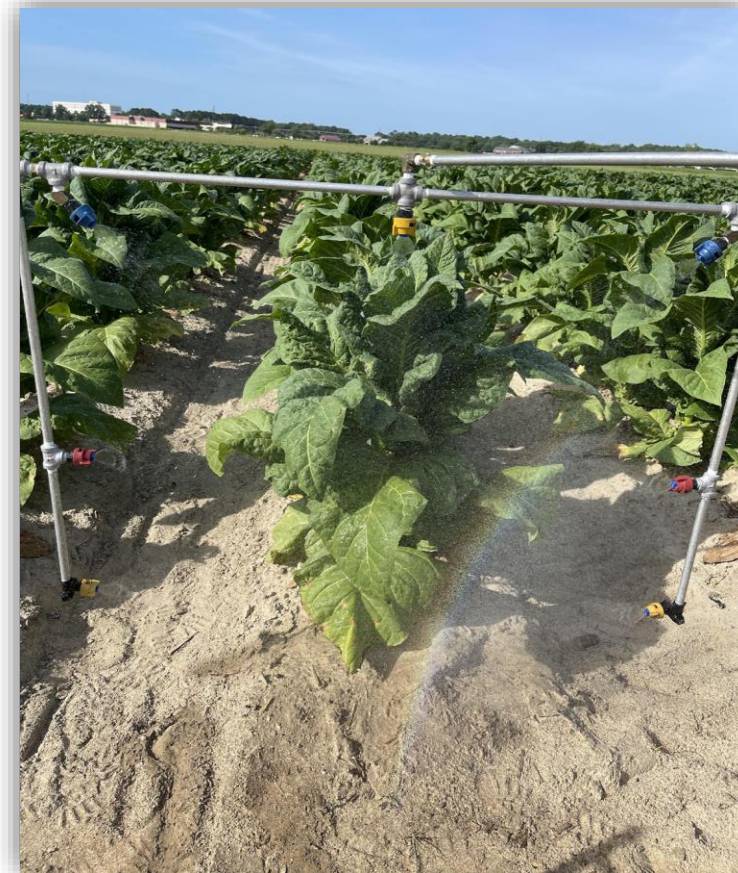
Drop Nozzle Application XR8003 - XR11003 (7) flat fan nozzles 50 GPA Output
