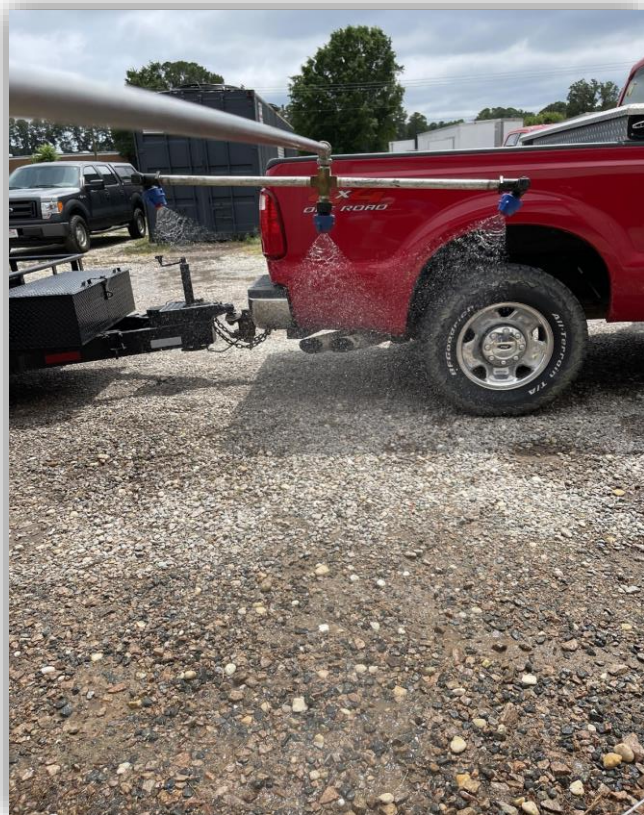
XR8004 Flat Fan Nozzles (3) 20 in. Boom Width 35 GPA Output
