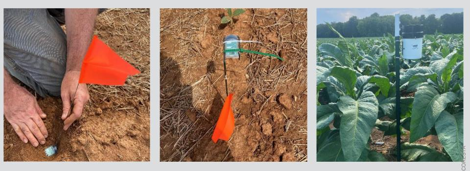
Soil temperature sensor buried 7.6 cm below soil surface, logged temperature every hour Air temperature sensor 30.5 cm above soil surface, logged temperature every hour, 15 cm soil sample Rain gauge placed at topping height, measured rainfall during growing season
