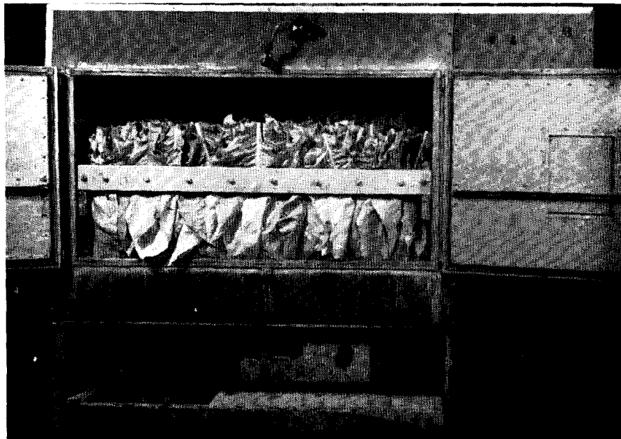
Figure 2. Climatic chamber used in the laboratory testing of bulk curing.
