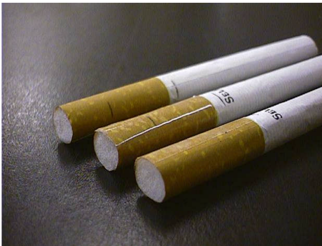
Figure 1. Example of 50% Vent Blocking
