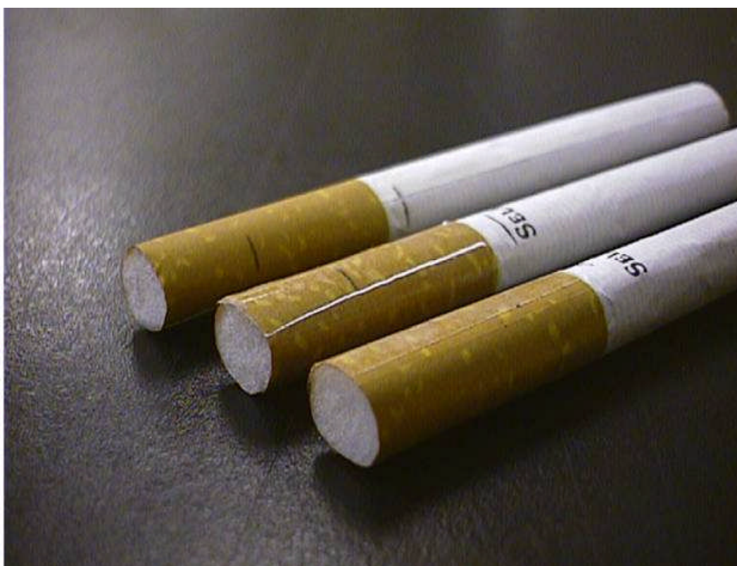
Figure 1. Example of 50% Vent Blocking
