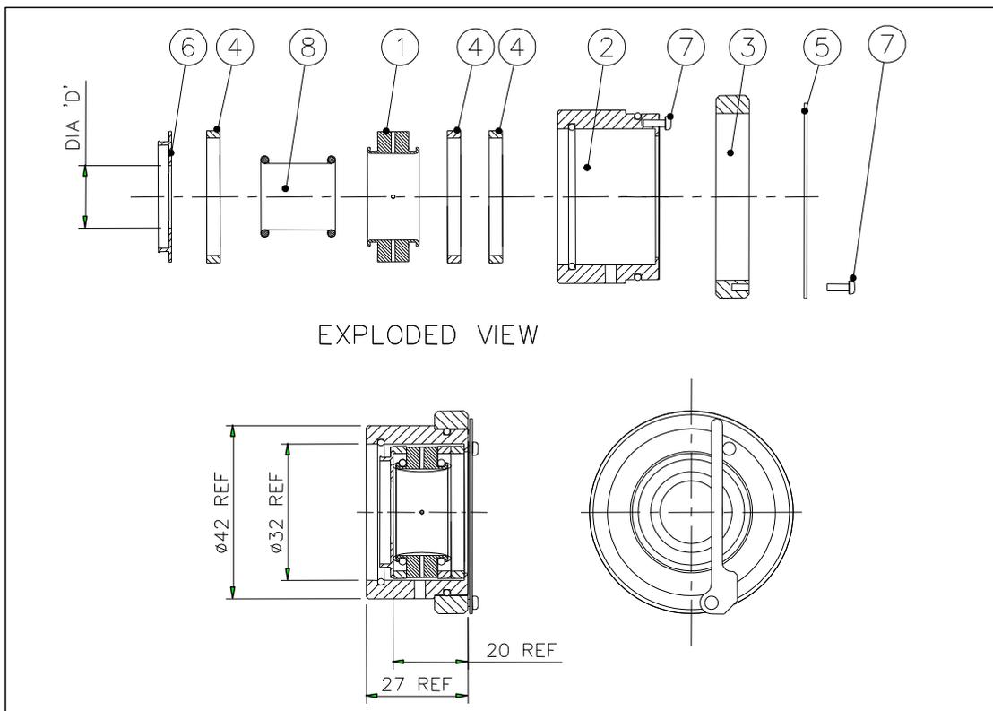
**Figure 4 - Example of Trap Assemblies for Cigars  $\varnothing$  6.5 to 16.49 mm and  $\varnothing$  16.5 to 22.5 mm**
