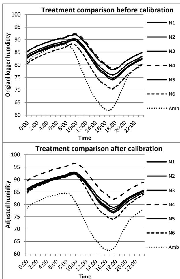
**Fig. 4. Twenty-four hour time plot of the mean humidity at various locations (N1 – N6) in a commercial barn over the duration of a cure of air-cured tobacco. A. Without adjusting for sensor accuracy drift. B. After logger calibration and adjustment for drift. Note especially the difference between the data for positions N4, N6 and Ambient.**
