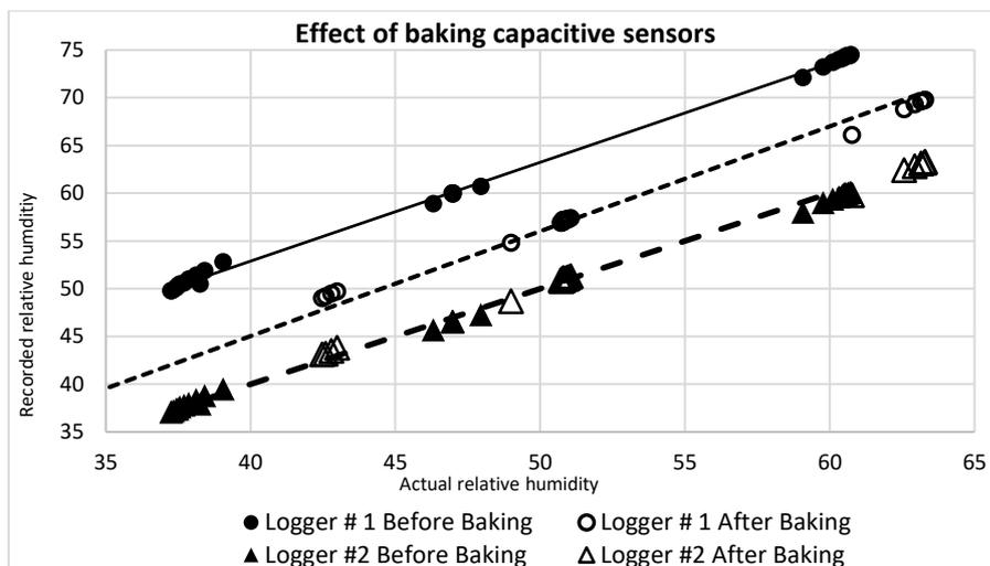
**Fig. 3. Baking capacitive sensors can decrease inaccuracy: Baking reduced the drift of logger # 1 from 13 % down to 6 %. It made no difference to Logger # 2 that was accurate to begin with.**
