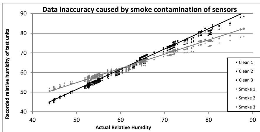
**Fig. 2. Smoke contamination of the sensors in loggers used in a fire-cured barn caused severe distortion of the recorded data.**
