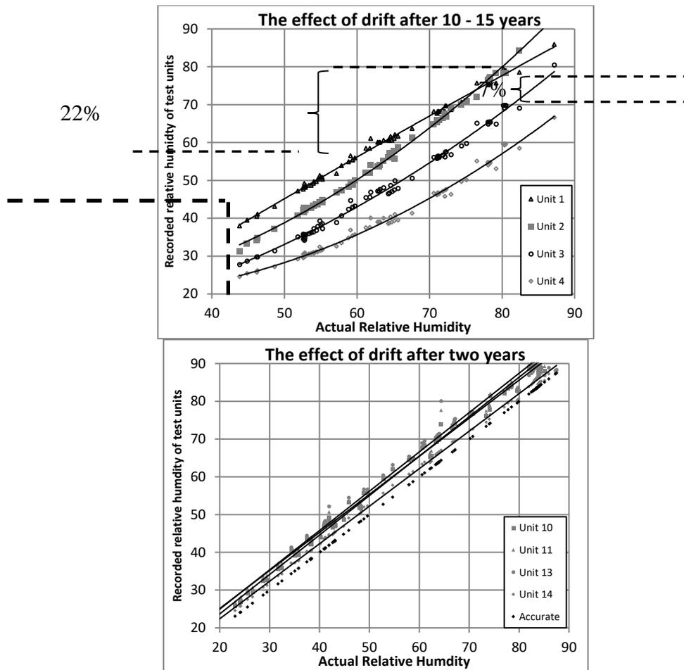
**Fig. 1. Accuracy drift of relative humidity sensors with time. A. Data from four data loggers over 10 years old varied by more than 20 % humidity between them and by as much as 25 % below the true humidity. B. Even after two years, there was at least a 5 % difference between loggers, and all were recording higher values than the actual humidity.**
